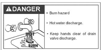
(4) Attach a hose to the water heater drain valve and put the other end in a floor drain or outdoors. Open the water heater drain valve. Open a nearby hot water faucet which will relieve pressure in the water heater and speed draining. The water passing out of the drain valve may be extremely hot. To avoid being scalded, make sure all connections are tight and that the water flow is directed away from any person, see Figures 2 and 5.
